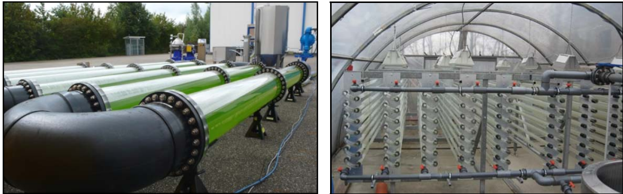
Figure 2. Tubular photobioreactors in outdoor (left) and enclosed (right) environments.
