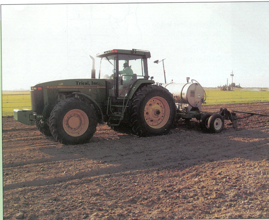
1,3-D is typically applied by custom applicators using a rig to inject the liquid into the soil, where it volatilizes into a gas.
